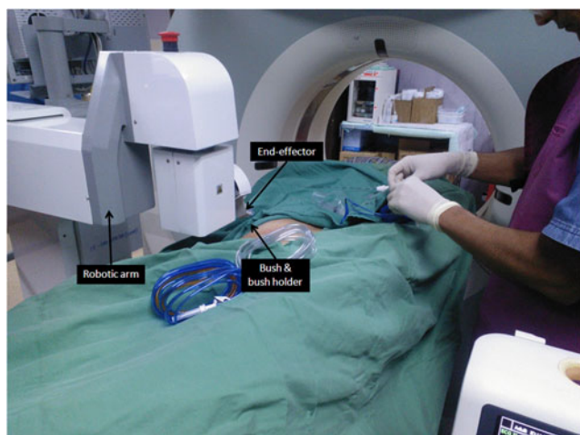
Fig. 2 The robotic arm was positioned automatically to the exact coordinates according to the treatment plan. The bush and bush holder were clamped firmly at the end-effector of the robotic arm before insertion of the RFA needle through the bush
